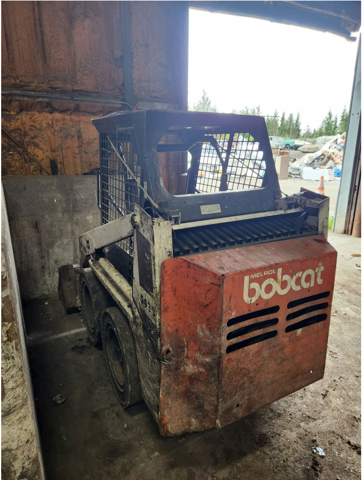
Current 31 year old skid steer loader – notice open cab and condition.
