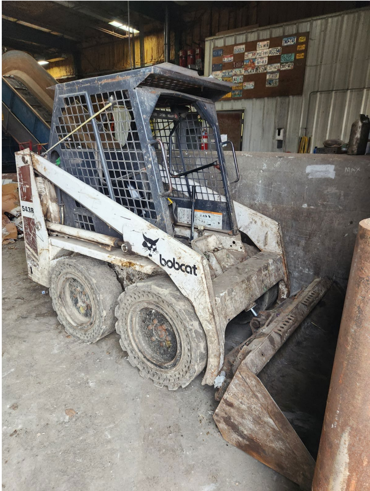
Another angle of the old worn out, 31 year old, skid steer loader – notice open cab and condition.
